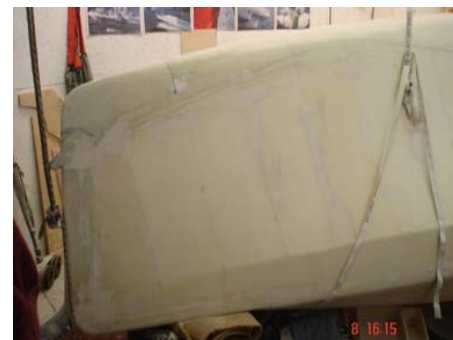
The bow (fibreglass over foam core) undergoing final preps
